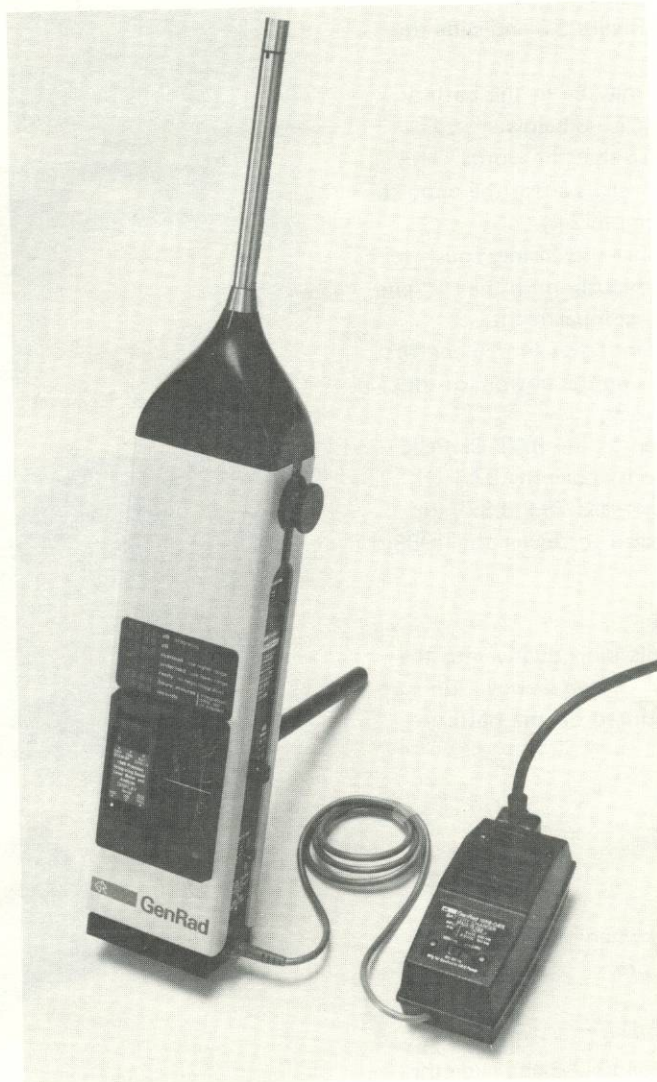
Figure 2-2. Proper connection of 1988-0411 Power Pack and Charger to 1988 battery-compartment jack. If the 1988 power switch is set to ON, 1988-0411 simultaneously powers the 1988 and recharges internal battery pack; if set to OFF, battery pack is recharged while 1988 power is disengaged.
